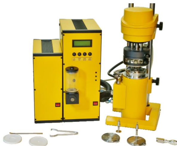
Figure 3 - Rheotest 4.1 Rotational viscosimeter, used for viscosity determination tests
